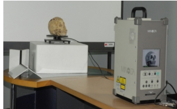
Figure 3: The set up of acquiring 3D model of the skull with the Vivid 910 3D Laser scanner
